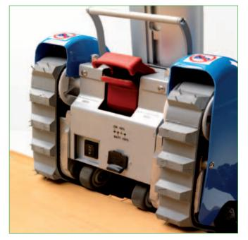
Double, electrical and mechanical lock, of the steering bar Tool for manual operation connection to the motor casing
