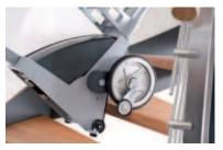
Mechanism for stopping at the step
